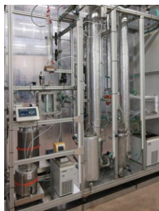
Bio-BTX scrubber unit (1 Nm 3 /h feed)
